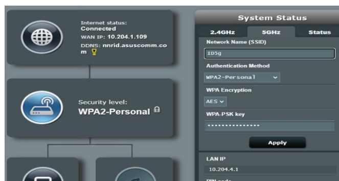
Gambar 10. Setup 5G and 2,4G routers
