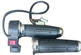
Gambar 3. Twist Throttle (www.indiamart.com)
